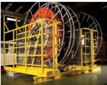
图示：旋转软管卷应用 Shown: Swivel in Hose Reel application
